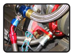
BECAUSE THE **JESEL** DISTRIBUTOR DRIVE KIT DOES NOT USE A PICK UP ASSEMBLY FOR THE IGNITION SYSTEM, A **CRANK TRIGGER** SETUP MUST BE USED WITH THE KIT. THE TIMING ADJUSTMENTS WILL NOW BE SET BY SLIDING THE CRANK TRIGGER BRACKET UP OR DOWN AS OPPOSED TO TURNING THE DISTRIBUTOR CLOCKWISE OR COUNTER-CLOCKWISE.
