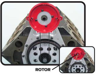
STEP 4: WITH THE FOUR ALLEN BOLTS TORQUED TO SPEC, YOU CAN INSTALL THE DISTRIBUTOR ROTOR. MAKE SURE THE ROTOR IS ALIGNED WITH THE NUMBER ONE SPARK PLUG TERMINAL AFTER THE NUMBER ONE CYLINDER IS AT TDC ON THE COMPRESSION STROKE. FROM THERE, THE TIMING CAN BE PHASED IN BY LOOSENING THE THREE BRACKET TO HOUSING BOLTS AND ROTATING THE DISTRIBUTOR HOUSING.
