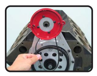
STEP 3: INSTALL THE JESEL DISTRIBUTOR DRIVE HOUSING ASSEMBLY (WHICH COMES ASSEMBLED FROM JESEL) WITH ONE BOLT ONLY AND LEAVE IT SLIGHTLY LOOSE. THIS WILL ENABLE YOU TO EASILY PLACE THE BELT OVER THE LOWER DRIVE GEAR. WITH THE BELT ENGAGED ON THE DRIVE GEAR TEETH, INSTALL THE REMAINING THREE ALLEN-HEAD BRACKET BOLTS AND TORQUE THEM TO 12 LBS-FT.
