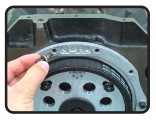
STEP 1: WHEN INSTALLING THE JESEL DISTRIBUTOR DRIVE ON AN ENGINE ALREADY EQUIPPED WITH A JESEL BELT DRIVE SYSTEM, BEGIN BY REMOVING THE TOP FOUR COVER BOLTS FROM THE BLOCK. WITH THE COVER BOLTS REMOVED, LOOSEN AND REMOVE THE CENTER LH THREAD CAM BOLT AND REMOVE THE CAMSHAFT ADAPTER WASHER FROM THE FRONT OF THE ENGINE. THERE IS AN INSTRUCTION SHEET INCLUDED WITH ALL JESEL BELT DRIVE SYSTEMS IF YOU ARE INSTALLING BOTH KITS AT THE SAME TIME.
