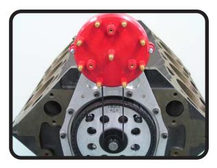
STEP 5: WITH THE INSTALLATION NEARING COMPLETION, YOU CAN INSTALL THE DISTRIBUTOR CAP AFTER THE ROTOR HAS BEEN PROPERLY PHASED. WITH THE CAP ON AND TIGHTENED DOWN, YOU CAN INSTALL THE EIGHT SPARK PLUG WIRES AND SET THE IGNITION TIMING TO SPEC BY MAKING MINOR ADJUSTMENTS AT THE CRANK TRIGGER PICKUP BRACKET BY THE HARMONIC BALANCER.
