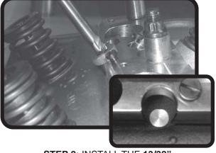
STEP 2: INSTALL THE 13/32" DRILL BUSHING INTO DRILL JIG. MILL HEAD USING SPOTFACE **CUTTER UNTIL THE SURFACE** IS CLEAN.
