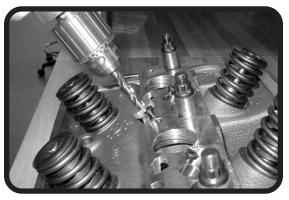
STEP 3: INSTALL "O" DRILL BUSHING, ZERO OUT VERNIER CALIPER FROM SPOTFACE SURFACE TO THE TOP OF THE DRILL BUSHING.
