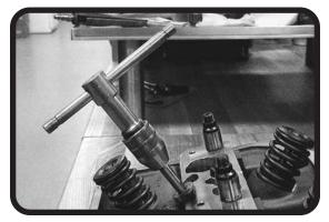
STEP 5: INSTALL "W" DRILL BUSHING AND TAP THE FRESHLY DRILLED HOLE BY FIRST USING THE 3/8-16 H2 HAND TAP FOLLOWED THE 3/8-16 H2 BOTTOMING TAP.
