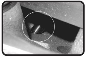
STEP 6: SCREW IN THE PROPER STUD THAT IS SUPPLIED IN THE ROCKER ARM KIT AND CHECK TO SEE THAT YOU HAVE FULL THREAD ENGAGEMENT.
